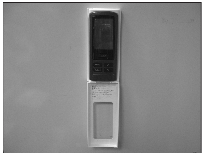
Figure 12.6 - Remote in Housing
