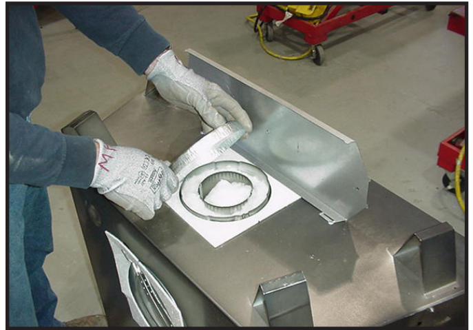
Figure 9.4 Remove the seal cap.
