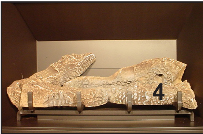
LOG #4 (SRV278-705): Position log #4 between log #1 and the locating tab on the fourth grate tine. Push its left hand side back to the locating tab as the grate tine.
