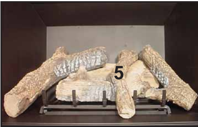
LOG #5 (SRV385-723): Position log #5 between the 3rd and 4th grate bar resting on the grooves in log #1 and log #2.
