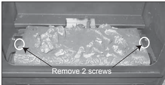
Figure 6.1 Remove top and front (if installed), glass, and logs (if installed). Remove burner by removing ONLY the two screws indicated. DO NOT remove the screws from the burner top. Lift the burner up and out of the firebox.
