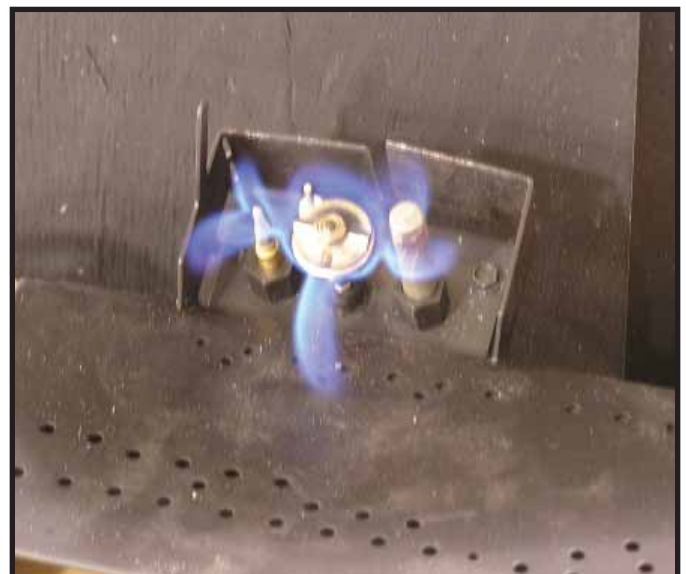
Figure 3.1 Standing Pilot Flame Patterns
