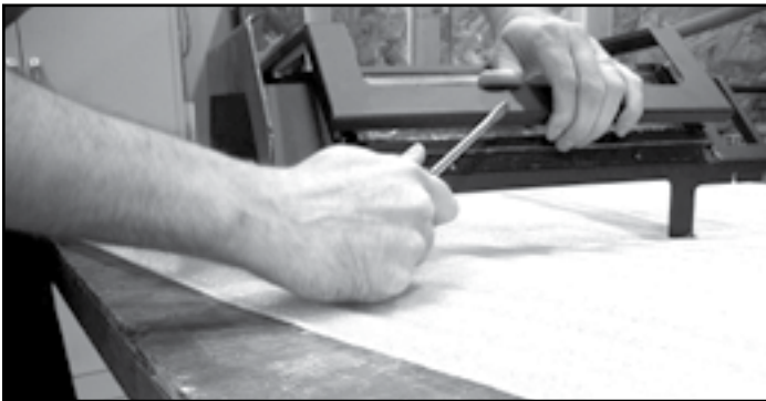
Figure 8.8 - Use a flat-head screwdriver to pry the black crown free on the right side. Remove the crown and discard.
