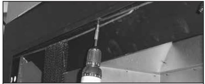
Figure 3.9 Removing the Screen Rods
