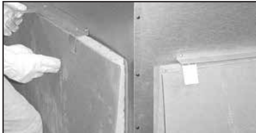
Figure 3.6 Unpacking Back Refractory
