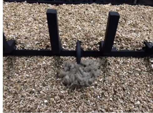
Figure 8a- Packing rock wool around the carry over tube
