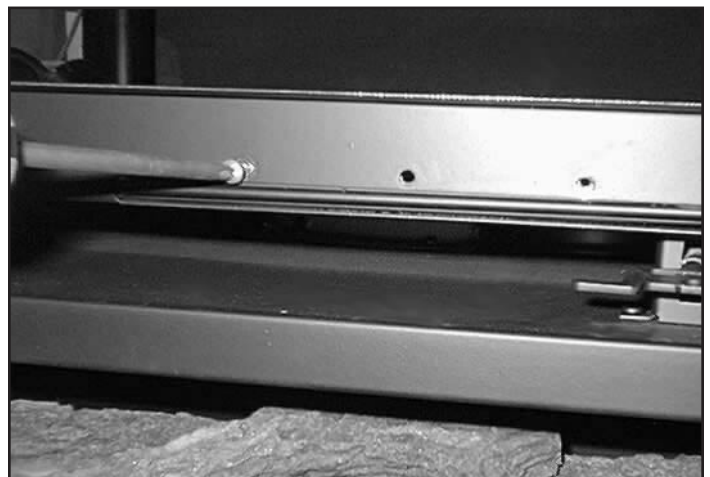
Figure 3 Removing the Starter Collar
