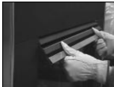
A - Removing the Upper Grille
