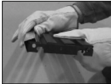
Figure 20 Putting Trim on Control Access Panel
