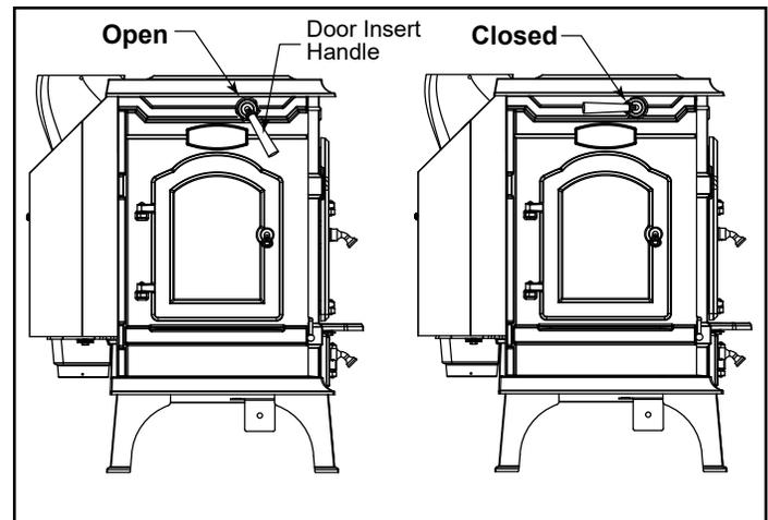
Figure 27 - Damper operating positions.
