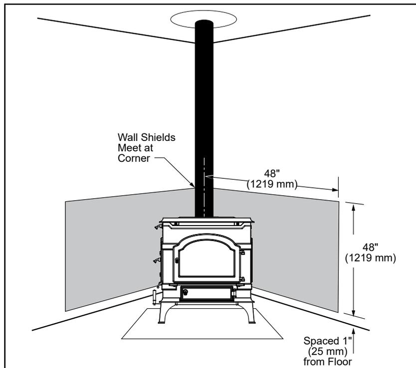
Figure 18 - Corner wall protection.
