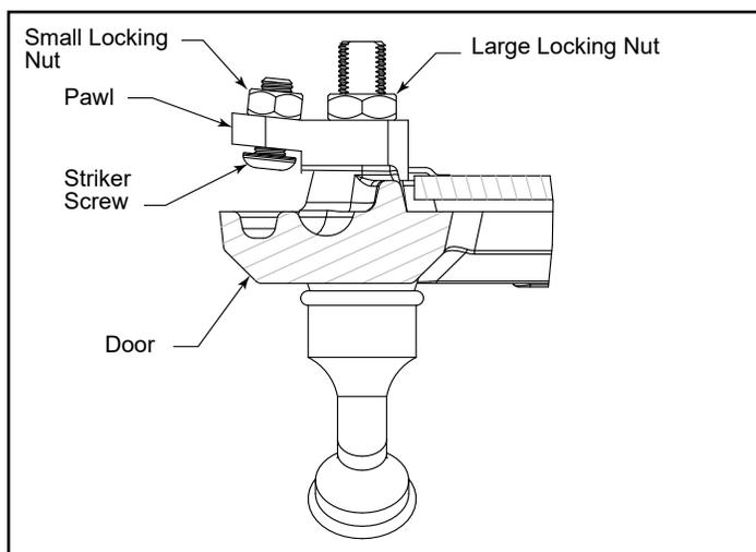
Figure 31 - Door latch adjustment.
