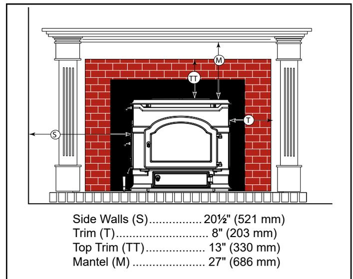
**Figure 15** - Minimum clearances for fireplace installation. Recommended clearances must be maintained between stove and the surrounding combustible components.
