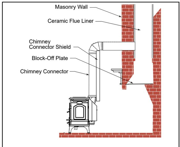
**Figure 8** - The connector enters flue above the fireplace. If the clearance between the chimney connector and either the mantel and/or the ceiling is inadequate, special protective shields will be required.
