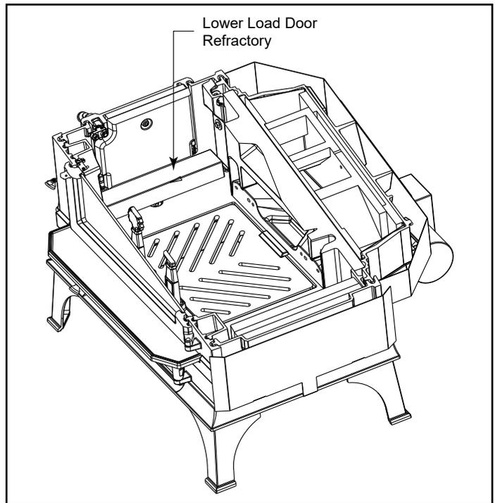
Figure 22 - Install lower load door refractory. (Cutaway view for clarification.)
