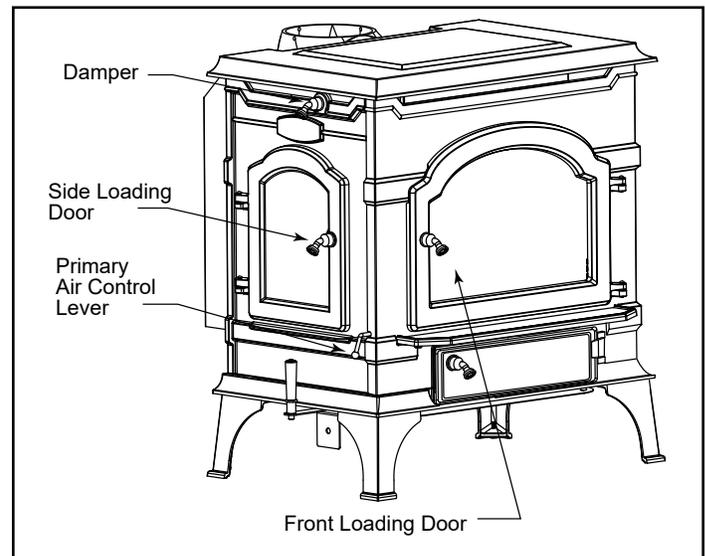
Figure 24 - The heater controls.
