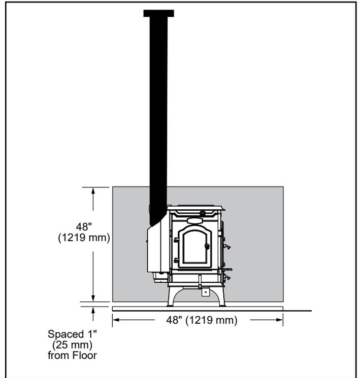
Figure 17 - Sidewall protection.
