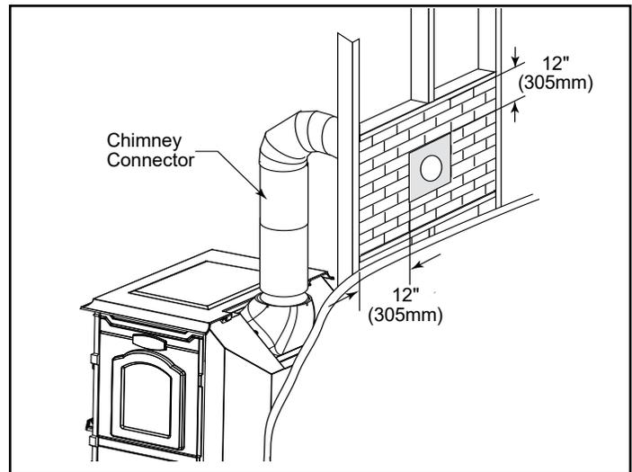
**Figure 10** - Wall pass-through enclosed with noncombustible materials.
