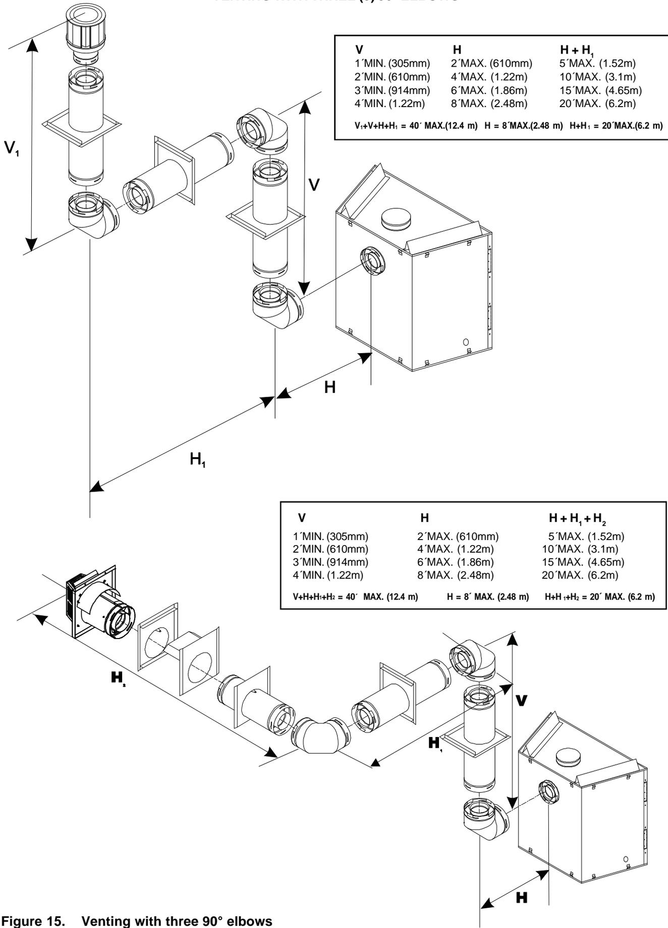
Figure 15. Venting with three 90° elbows
