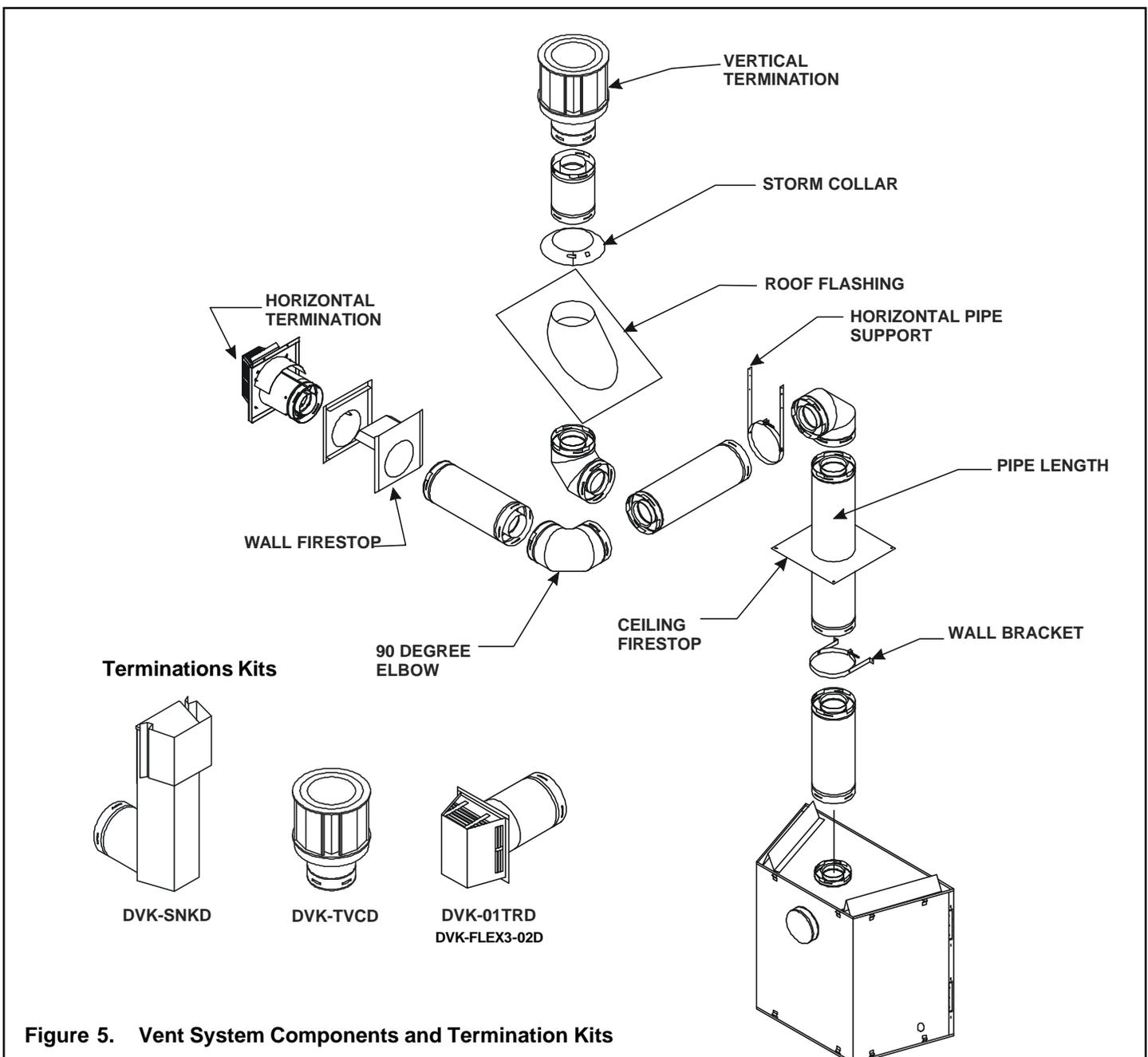
Figure 5. Vent System Components and Termination Kits
