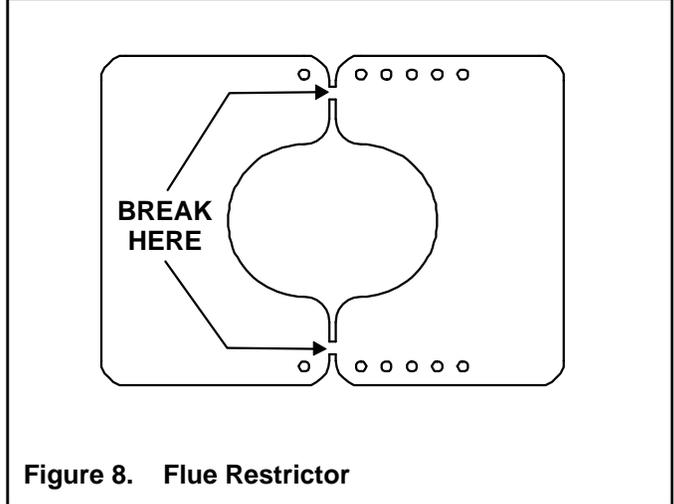
3. Match the amount of vertical you have in the system with the chart to find the appropriate position to set the Flue Restrictor.
