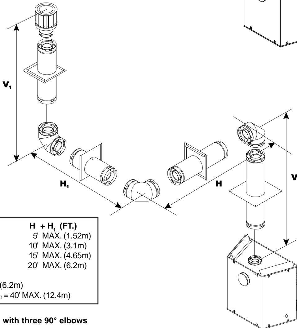
**Figure 16. Venting with three 90° elbows**
