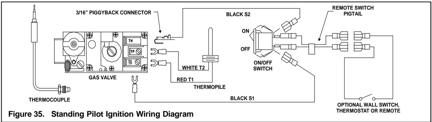
Figure 35. Standing Pilot Ignition Wiring Diagram
