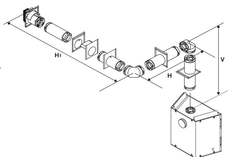
Figure 14. Venting with Two 90° Elbows
