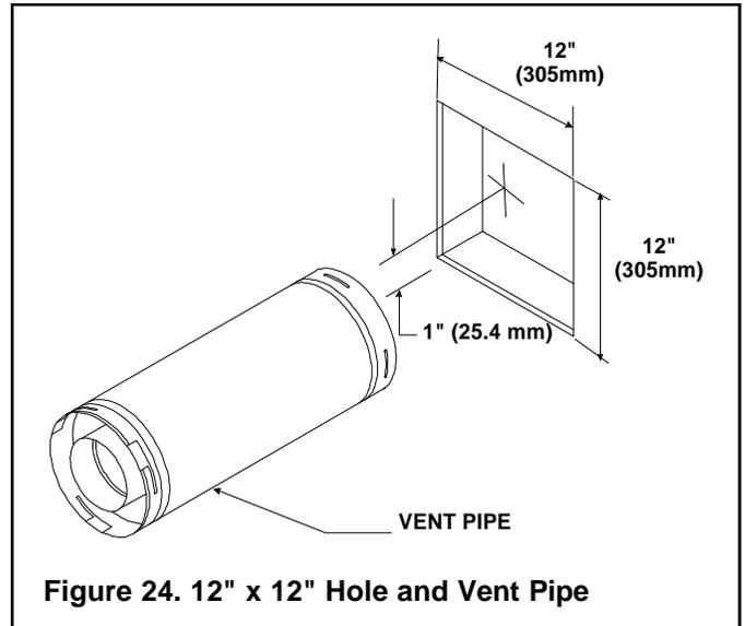
Figure 24. 12" x 12" Hole and Vent Pipe
