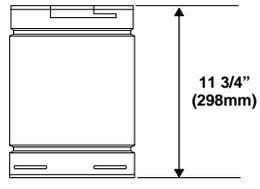
**NOTE: PIPES OVERLAP 1-3/8 INCHES (34.93mm) AT EACH JOINT.**
