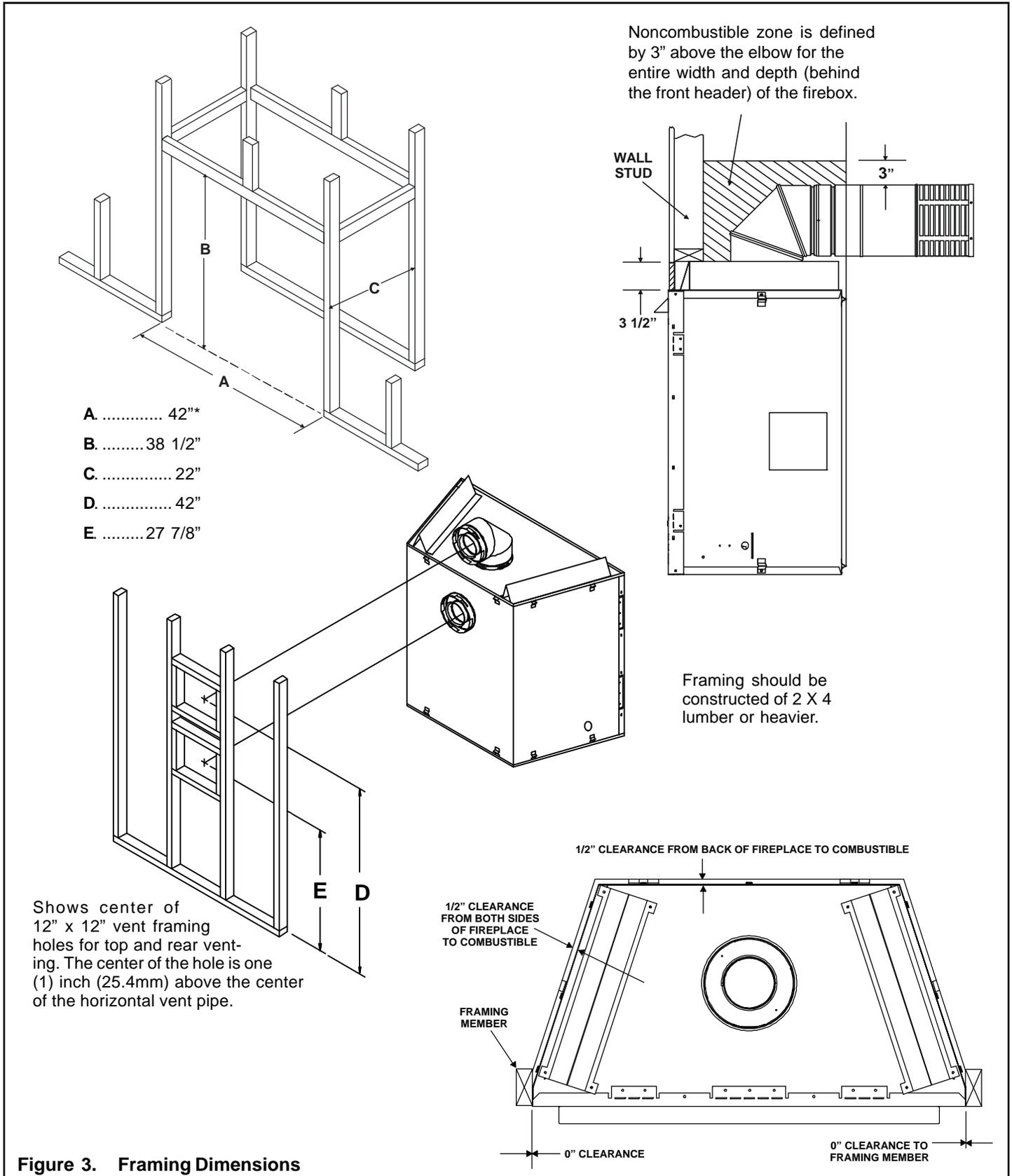
Figure 3. Framing Dimensions
