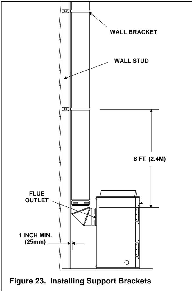
Figure 23. Installing Support Brackets
