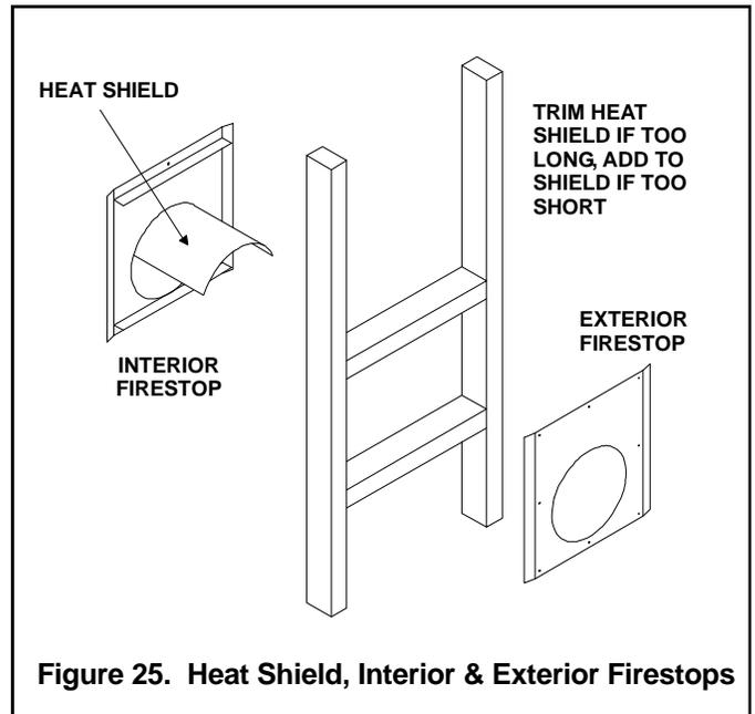
Figure 25. Heat Shield, Interior & Exterior Firestops
