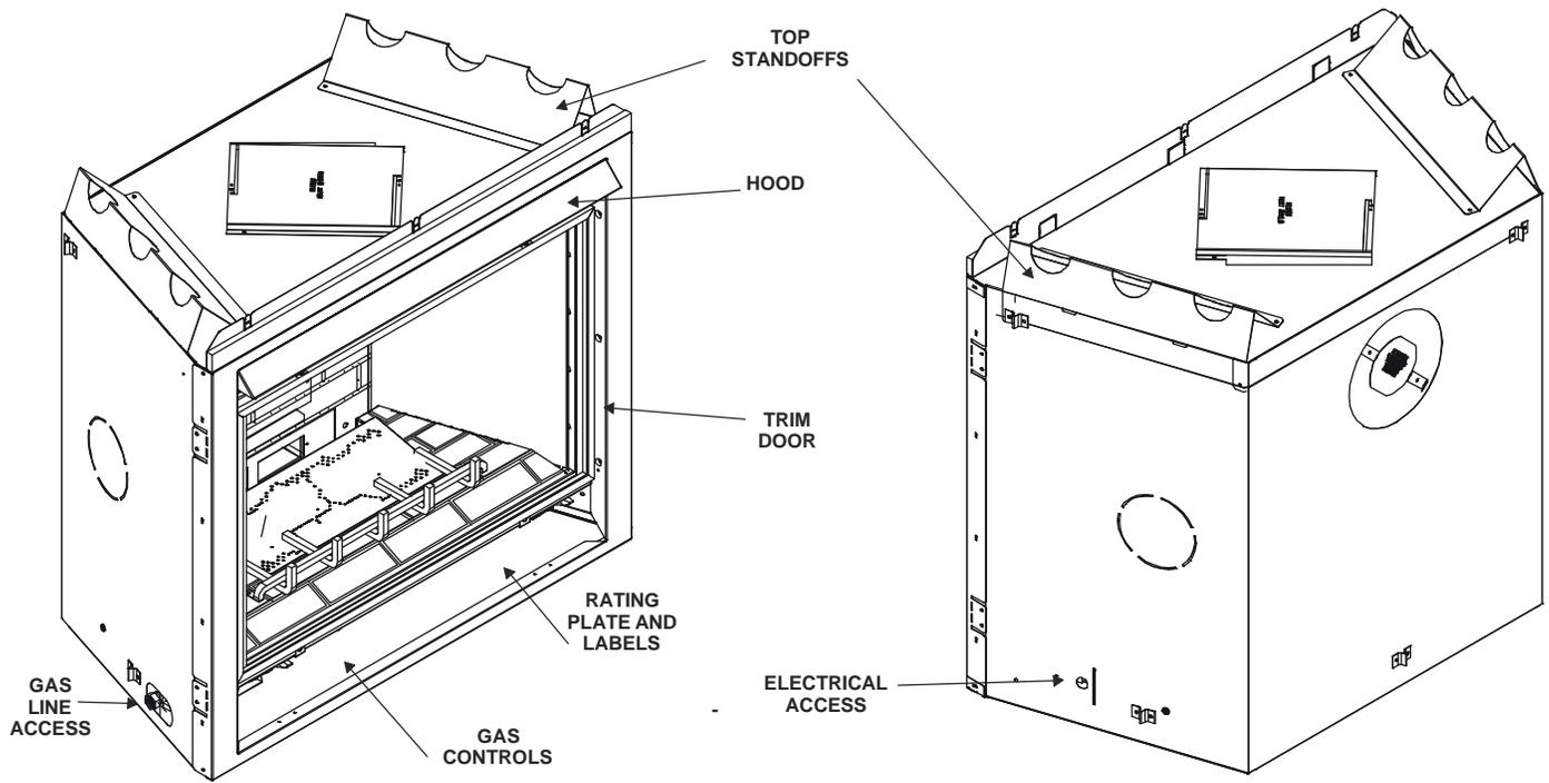
Figure 1. Diagram of the QV36D
