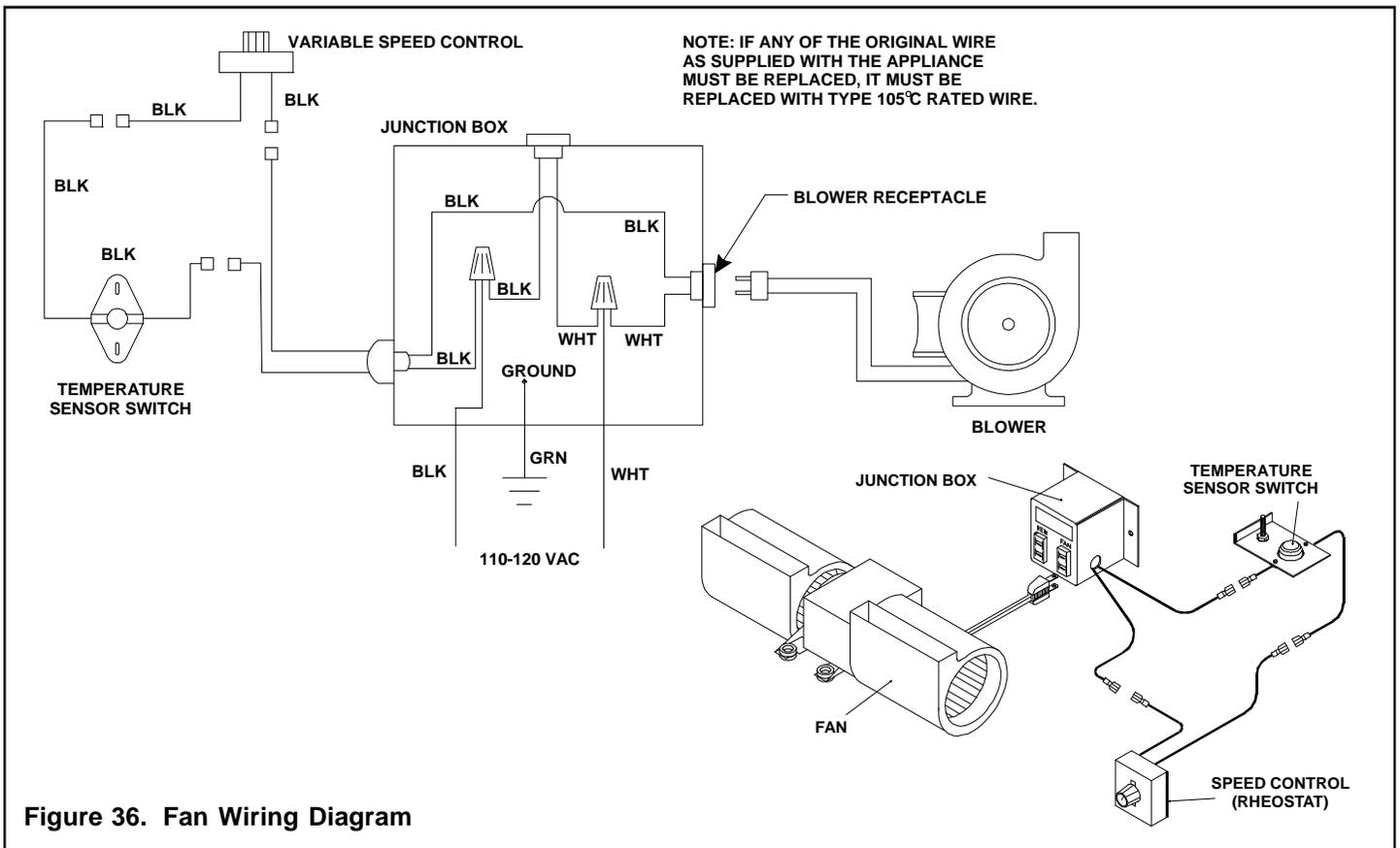
Figure 36. Fan Wiring Diagram
