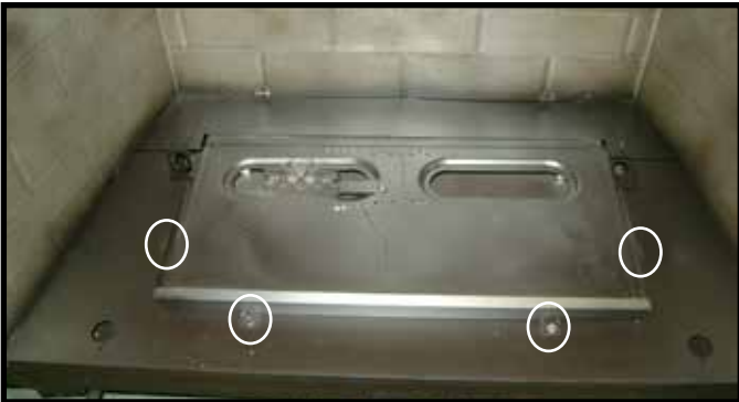
Figure 4.10 Remove Burner Skirt
