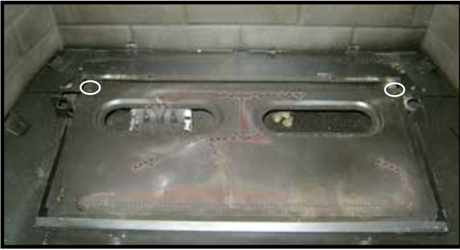
Figure 4.9 Remove Screws from Burner Assembly Rear Corners
