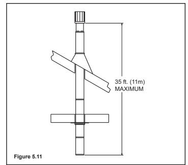
**NOTE:** Maximum number of 90° elbows permitted for a vertical installation is four, provided the termination falls within the shaded area shown in vent graph on page 10. See also **Figure 5.12**, within the four 90° elbows configuration, the maximum allowable pipe length on the horizontal runs is 1 ft. (305mm) the minimum allowable pipe length on vertical runs is 1 ft. (305mm).
