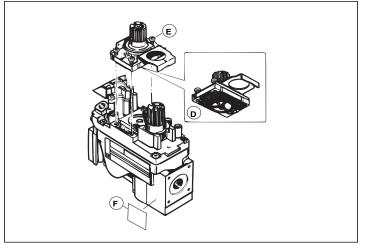
**Figure 6.6** Ensure that the rubber gasket (**D**) is properly positioned and install the new HI/LO pressure regulator assembly to the valve using the new screws (**E**) supplied with the kit. Tighten screws securely. (Reference torque = 25 in./lb.) Install the enclosed identification label (**F**) to the valve body where it can be seen.
