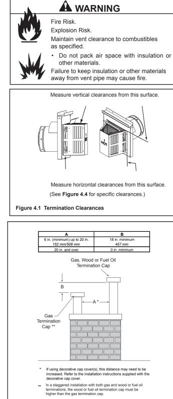
Figure 4.2 Multiple Vertical Termination
