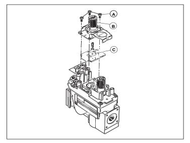
**Figure 6.5** Turn control knob to the OFF position, ensure that gas supply to the valve has been turned off. Using a Torx TH20, or slotted screwdriver, remove the three pressure regulator mounting screws (**A**), pressure regulator tower (**B**), and diaphragm (**C**).
