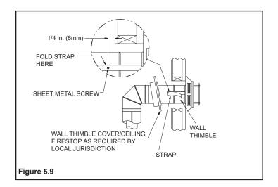
**Note:** The attachment from the vent pipe to the vent termination cap must be sealed with silicone with a minimum of 300°F continuous exposure rating. Termination caps shall not be recessed into a wall or siding.
