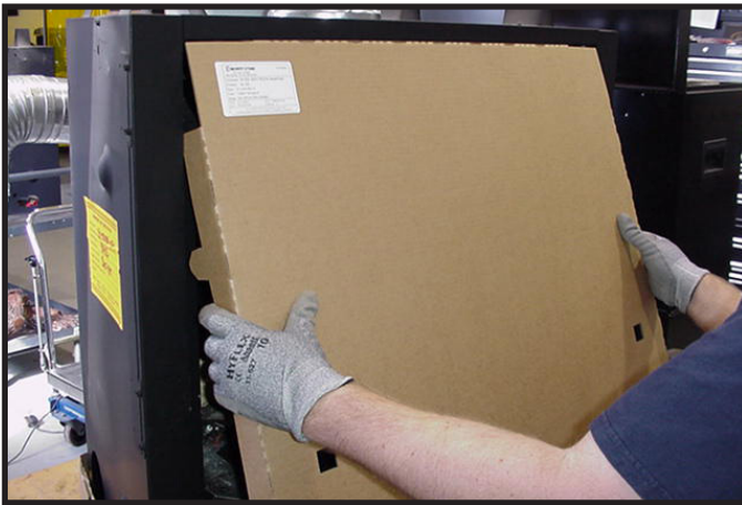
Figure 11.5 Installation of Splatter Guard
