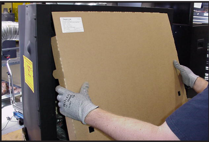
Figure 11.5 Installation of Splatter Guard
