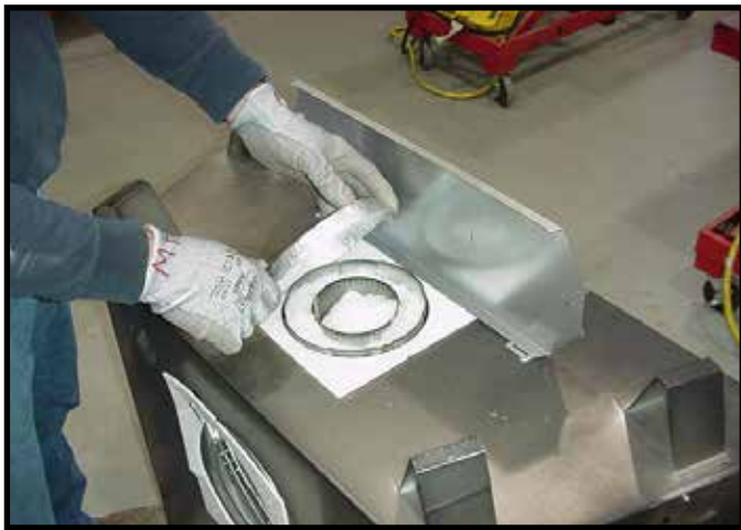
Figure 6.8 Remove the seal cap.
