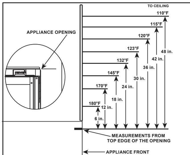
Figure 2.1 Maximum Wall Surface Temperatures Above Appliance
