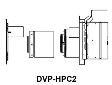
Figure 12.2 DVP Vent Components
