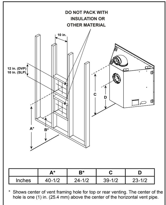
Figure 5.2 Wall Penetration
