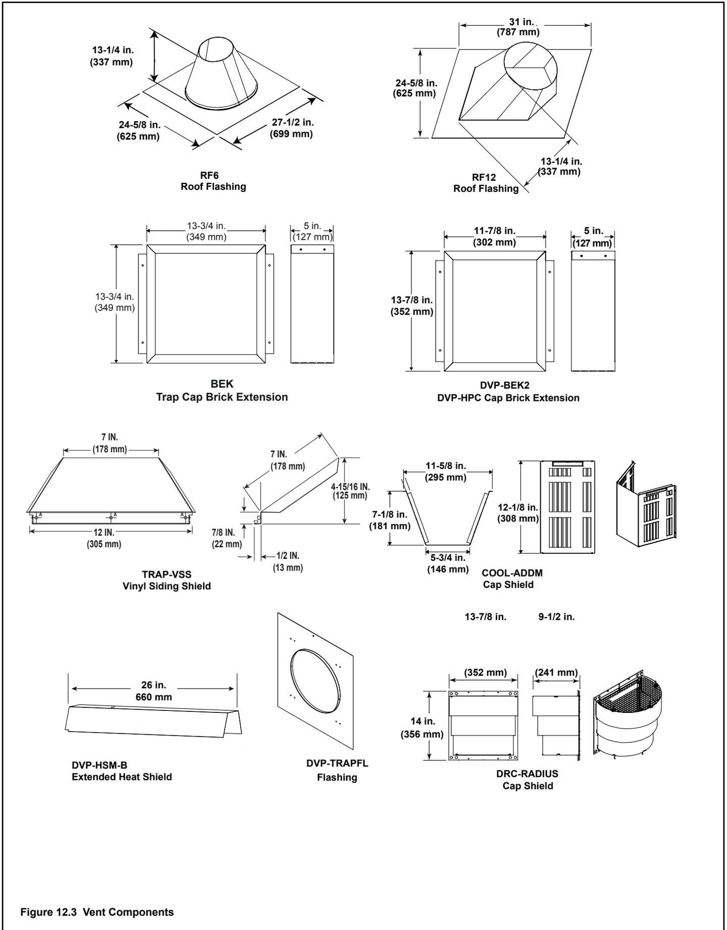
Figure 12.3 Vent Components
