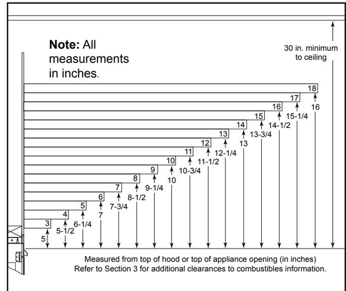
**Figure 10.1 Minimum Vertical and Maximum Horizontal Dimensions**
