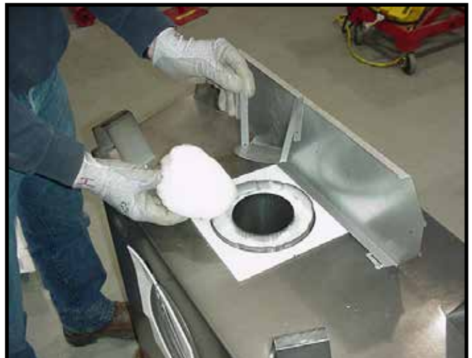
Figure 6.5 Remove the insulation basket and white insulation from the center vent pipe.
