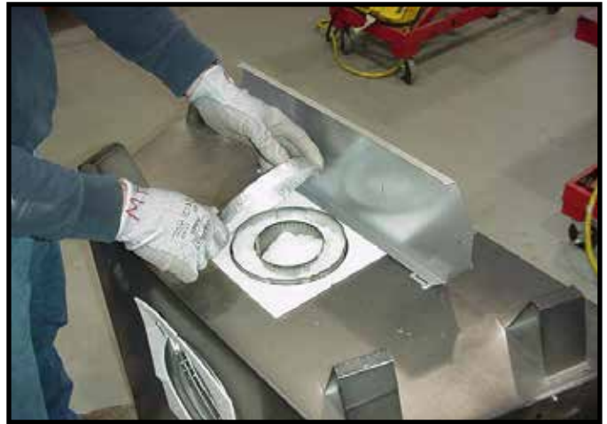
Figure 6.4 Remove the seal cap.
