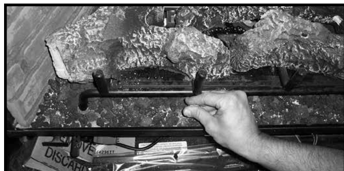
Figure 14.4 Placement of Vermiculite
