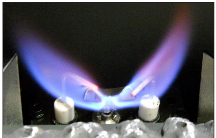
Figure 4.3 IPI Pilot Flame Patterns
