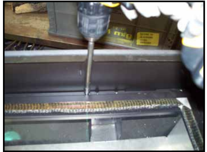
Figure 9.4. Gas and Electrical Access - Remove Glass Window
