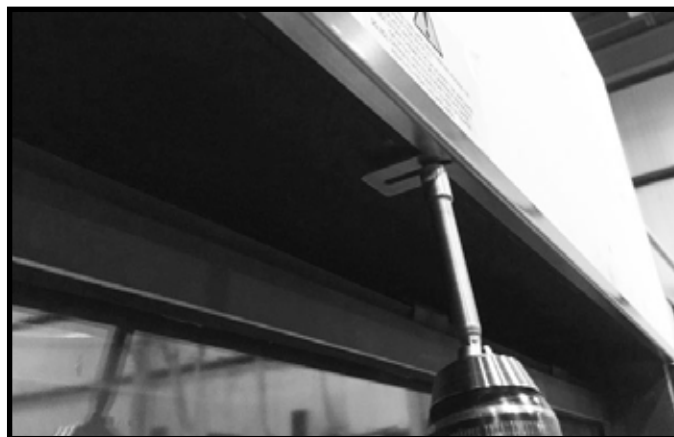
Figure 10.5. Install Trim Ring
