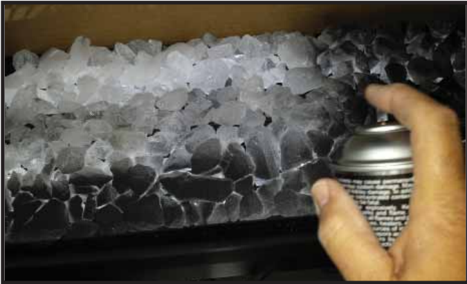
Figure 11.10 Fogging the Media
