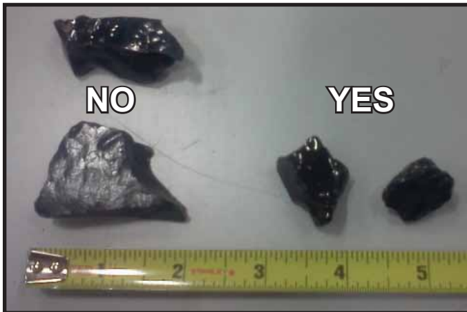
Figure 11.3. Selecting Flat Media for Pilot Cover.
