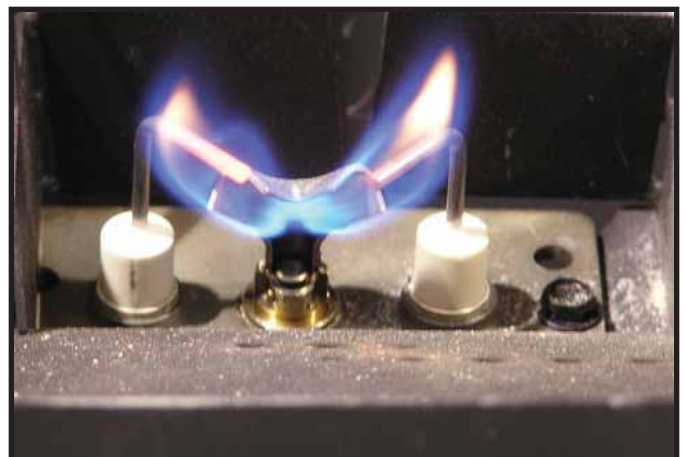
Figure 4.2 IPI Pilot Flame Patterns
