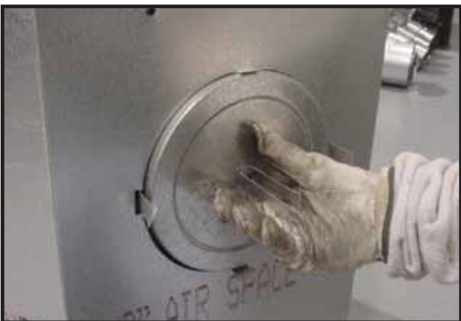
Figure 6.9 Fold the center parts of the retaining band toward the center as shown. Remove the seal cap.
