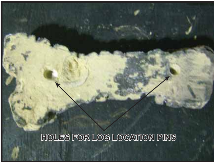
Figure 7. Log #3 Bottom View
