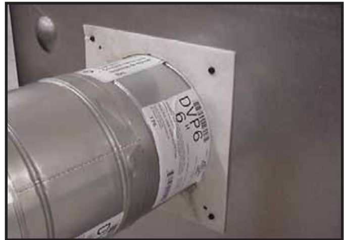
Figure 6.11 Attach the first vent section (it will snap into place). Slide the insulation gasket onto the vent section, up against the appliance and over the tabs. Use four self-tapping screws to secure gasket to outer wrap.
