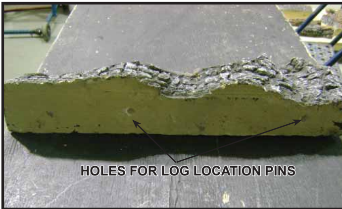
Figure 3. Log #1 - Bottom View
