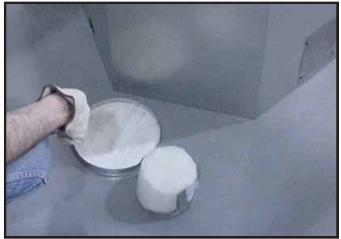
Figure 6.10 Discard the seal cap, remove and discard the insulation basket. Note: Once the seal cap has been removed it CANNOT be reattached.
