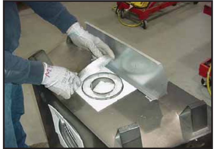
Figure 6.4 Remove the seal cap.
