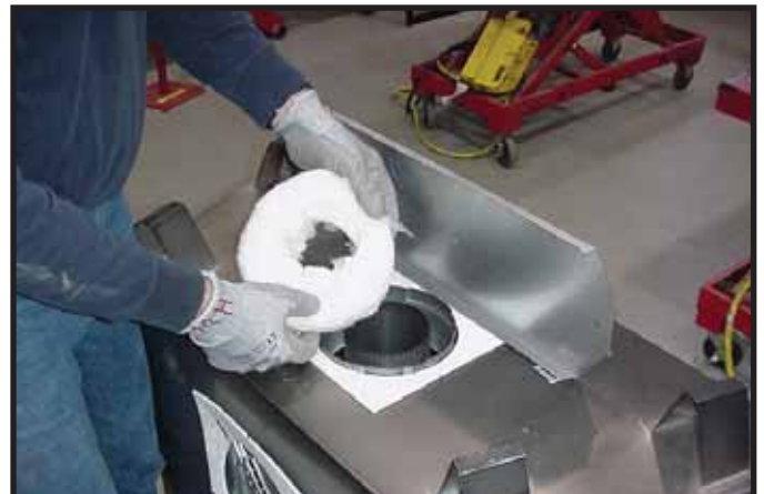
Figure 6.6 Remove the insulation from the outer vent pipe.
