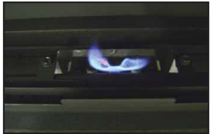
Figure 3.1 IPI Pilot Flame Pattern
