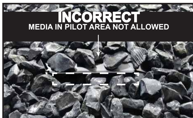
Figure 9.7 INCORRECT Media Placement
