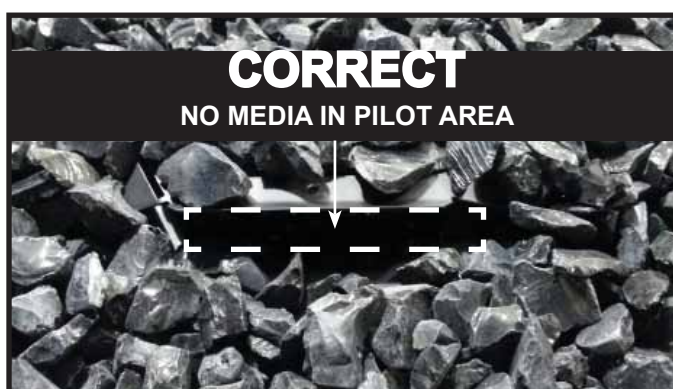
Figure 9.6 CORRECT Media Placement
