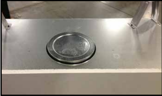
Figure 6.1 Seal Cap in Position
