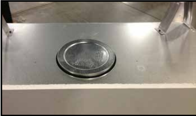
Figure 9.1 Seal Cap in Position
