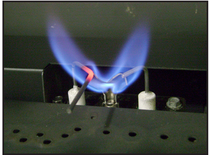
Figure 3.2 IPI Pilot Flame Patterns
