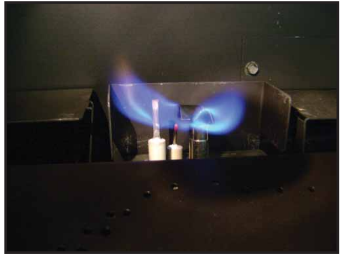
Figure 3.1 IPI Pilot Flame Patterns
