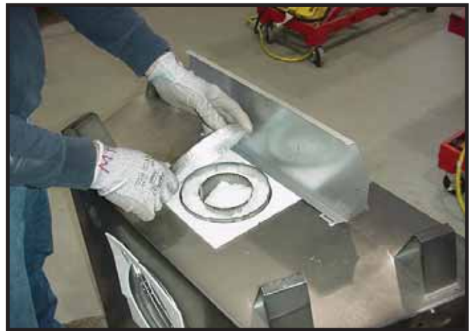
Figure 9.4 Remove the seal cap.
