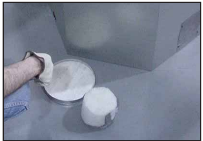
Figure 9.11 Discard the seal cap, remove and discard the insulation basket.
