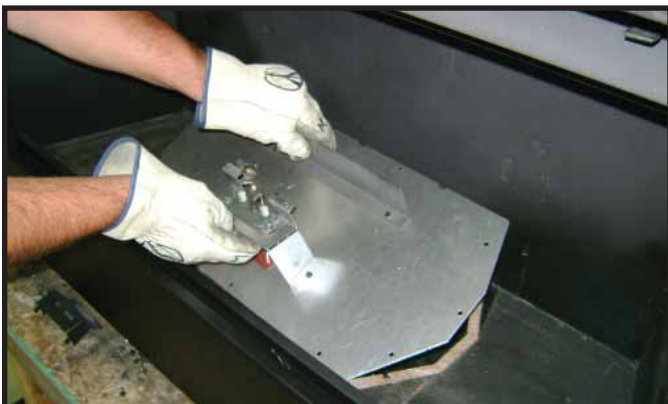
Figure 11.3. Remove Valve Plate
