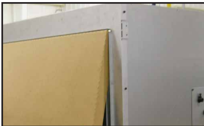
Figure 15.5 Splatter Guard Installation
