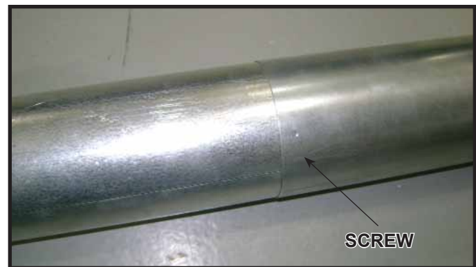
Figure 10.4 Screws into Slip Section
