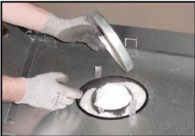
Figure 9.3 Remove the seal cap.
