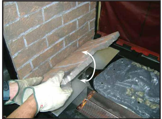
Figure 14.16 Positioning Inner Bottom Refractory
