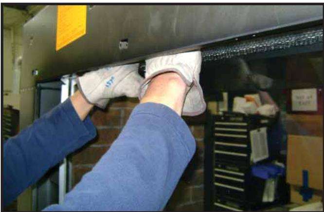
Figure 14.6 Top Glass Latch Access
