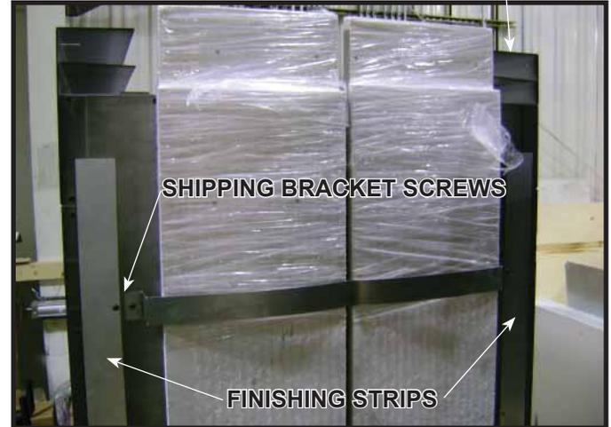
Figure 9.3 Shipping Brackets and Finishing Strip Locations.
