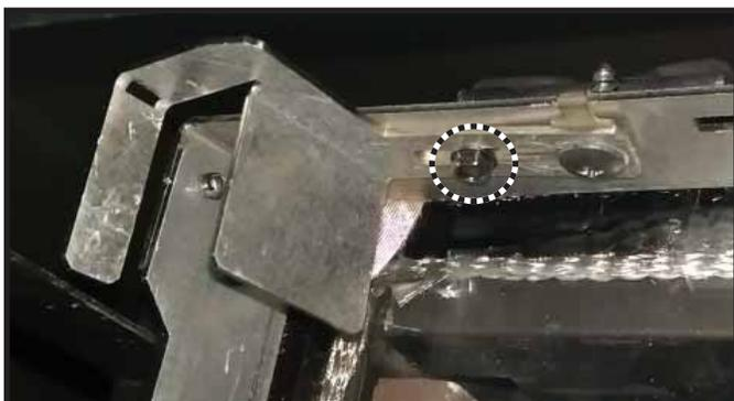
→ Figure 14.24 Shipping Location of Refractory Brackets
