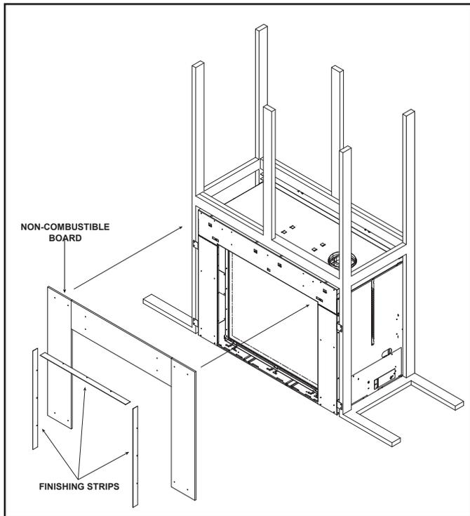
Figure 9.6 Attaching Non-Combustible Board
