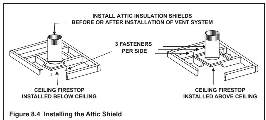
Figure 8.4 Installing the Attic Shield
