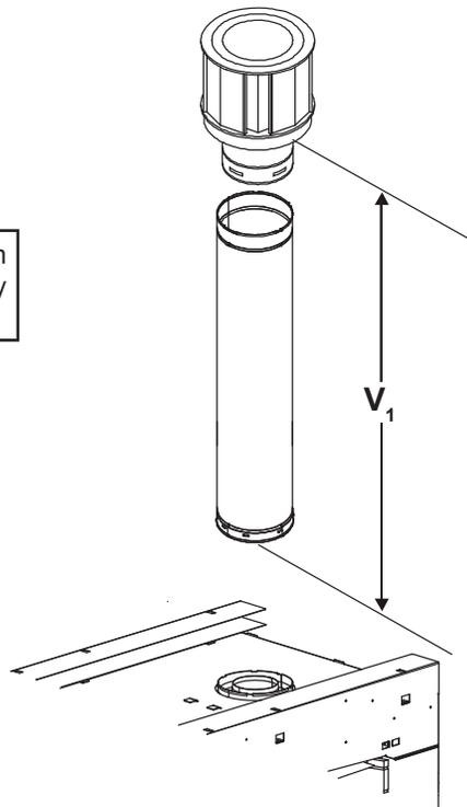
$V_1 = 50 \text{ ft. Max. (15.2 m)}$
