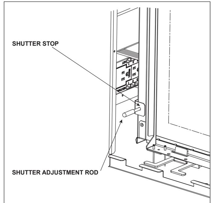
Figure 14.28 Shutter Adjustment Rod and Shutter Stop
