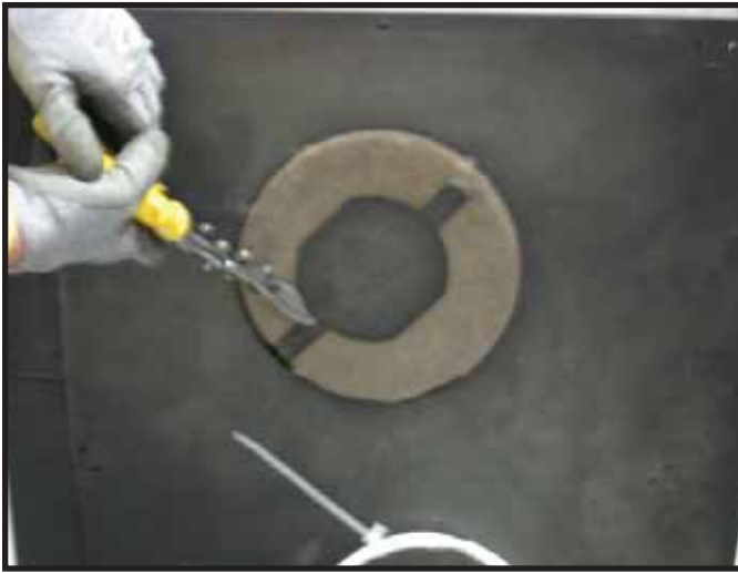
Figure 9.6 Cut the metal retaining band.
