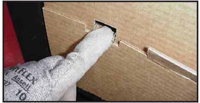
Figure 13.9 Securing Tabs Inside Front of Splatter Guard
