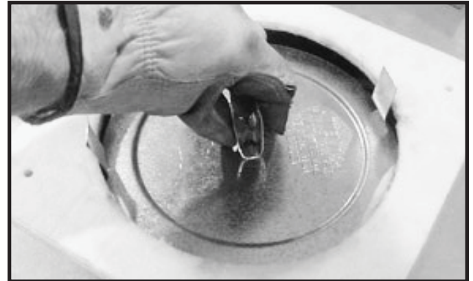
Figure 9.4 Fold the center parts of the retaining band and use to remove the vent cap.
