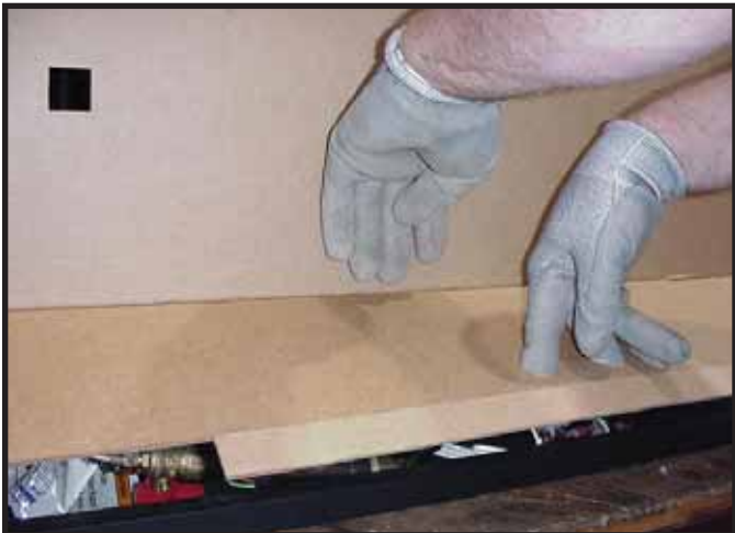
Figure 13.8 Opening Lower Access Panel
