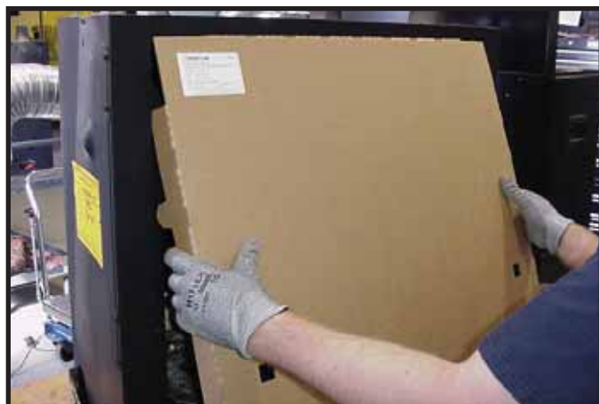
Figure 13.4 Installation of Splatter Guard
