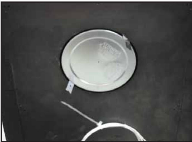
Figure 9.7 Remove the seal cap.
