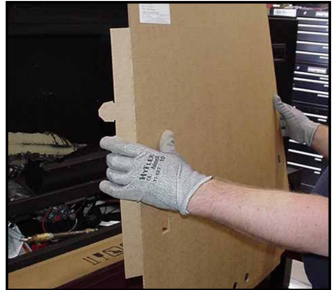
Figure 13.7 Folding of Right and Left Sides of Splatter Guard
