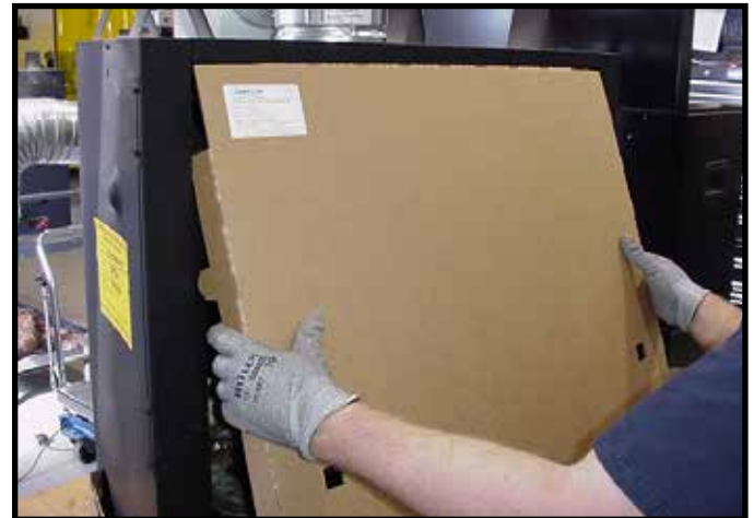
Figure 13.8 Installation of Splatter Guard
