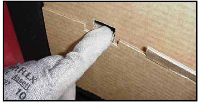
Figure 13.13 Securing Tabs Inside Front of Splatter Guard
