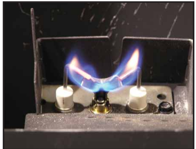
Figure 3.1 IPI Pilot Flame Patterns
