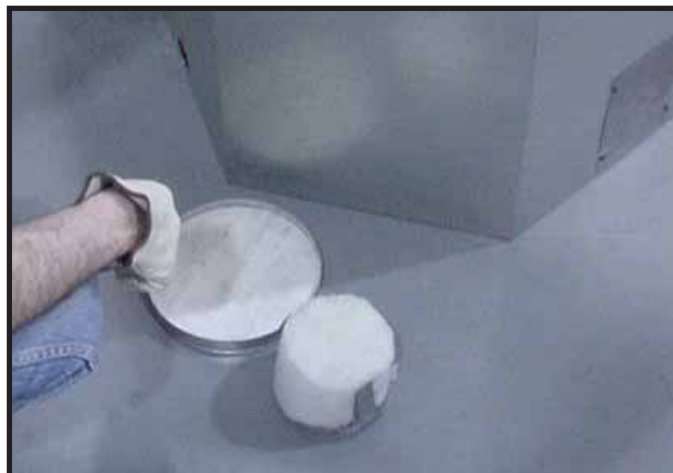
Figure 6.11 Discard the seal cap, remove and discard the insulation basket. Note: Once the vent cap has been removed it CANNOT be reattached.
