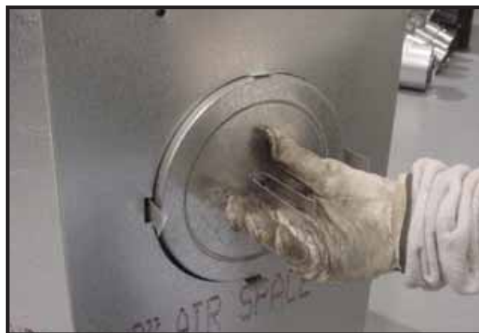
Figure 6.10 Fold the center parts of the retaining band out and use to remove the seal cap.
