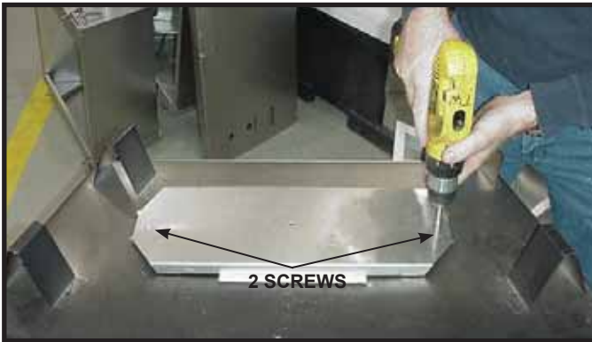
Figure 6.1 For top vent, remove the two screws holding the top heat shield in place. For rear vent, see Section 6.B.
