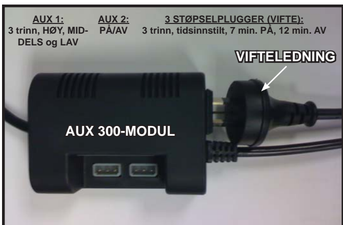
Fig. 12.10 Plugg viften inn i AUX300CE-modulen
