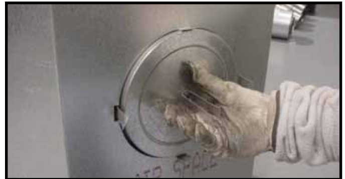
Figure 25. Fold the center parts of the retaining band out and use to remove the flue cap.
