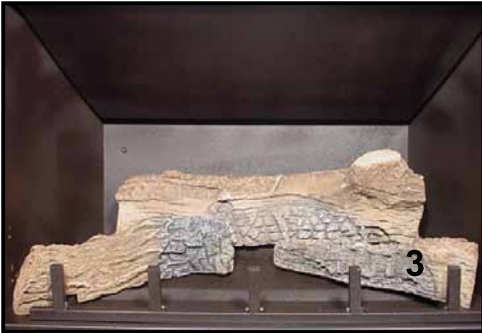
LOG #3 (SRV705-703): Rest log #3 against the right front grate corner and place its slot over the right burner tab.
