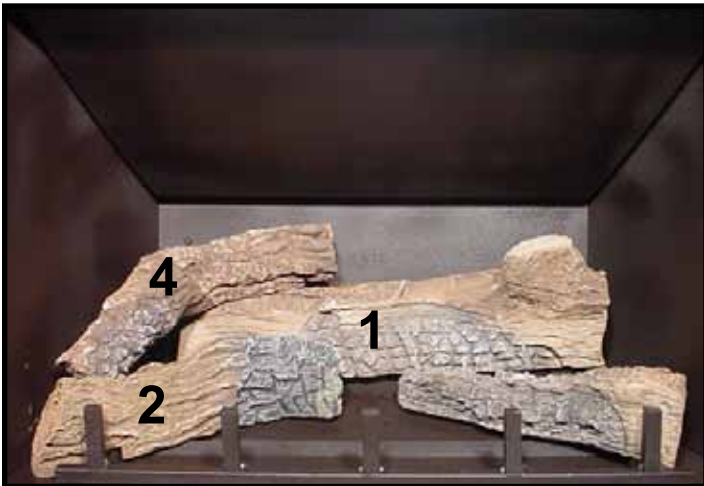
LOG #4 (SRV530-716): Place the left end of log #4 in the groove on log #2 and the right end on log #1 as shown.
