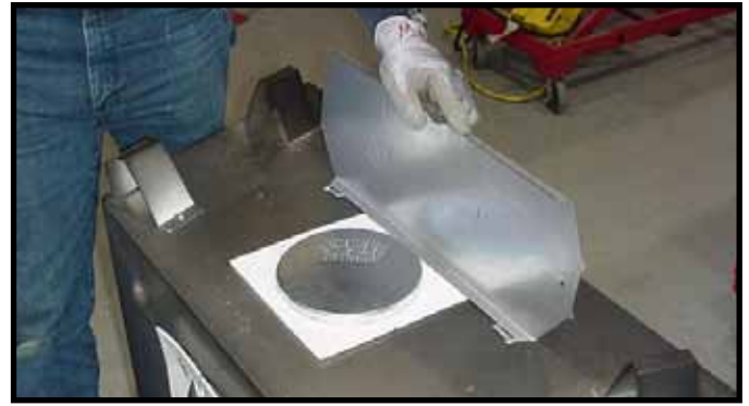
Figure 17. Rotate the top heat shield to the vertical position as shown above. The heat shield must remain in the vertical position.
