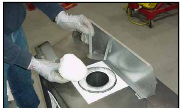
Figure 20. Remove the insulation basket and white insulation from the center flue pipe.
