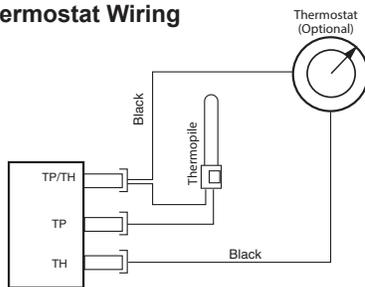
Figure 62 - On/Off switch and optional thermostat circuit.
