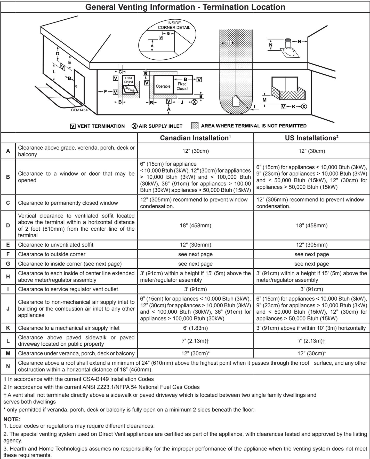
Figure 9 - Vent termination clearances.
