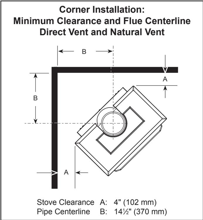
**Figure 4** - Corner installation, minimum corner clearances and flue centerline.
