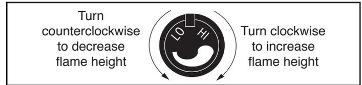
Figure 47 - Flame adjustment knob for Honeywell valve.
