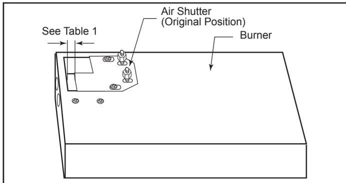
Figure 38 - Air shutter in original from-the-factory position.
