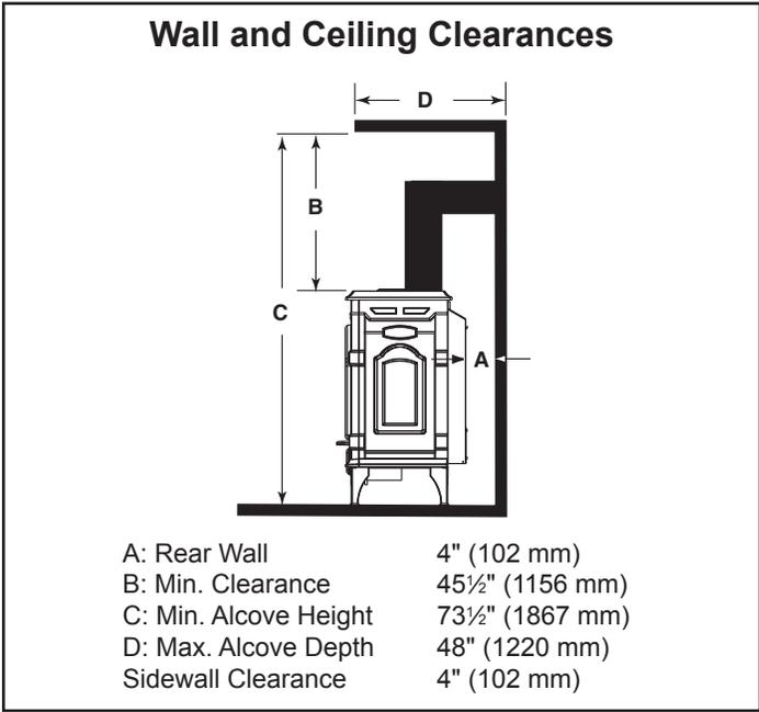
**Figure 6** - Dimensions and clearances to ceiling or alcove.
