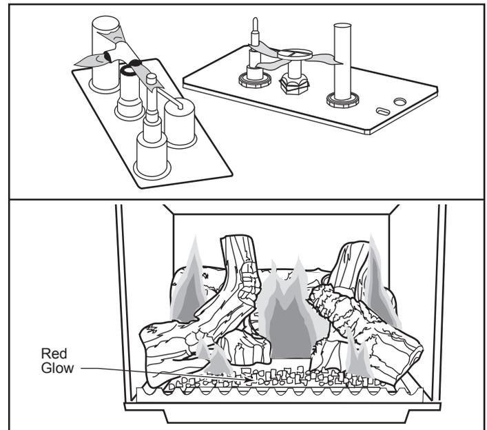
Figure 48 - Correct pilot and burner flame patterns.
