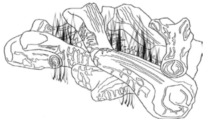
Figure 66 - Burner Flame Appearance
