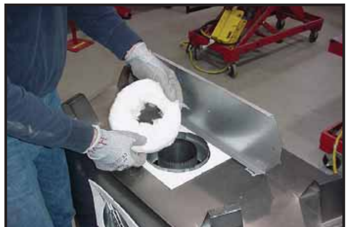
Figure 9.6 Remove the insulation from the outer vent pipe.
