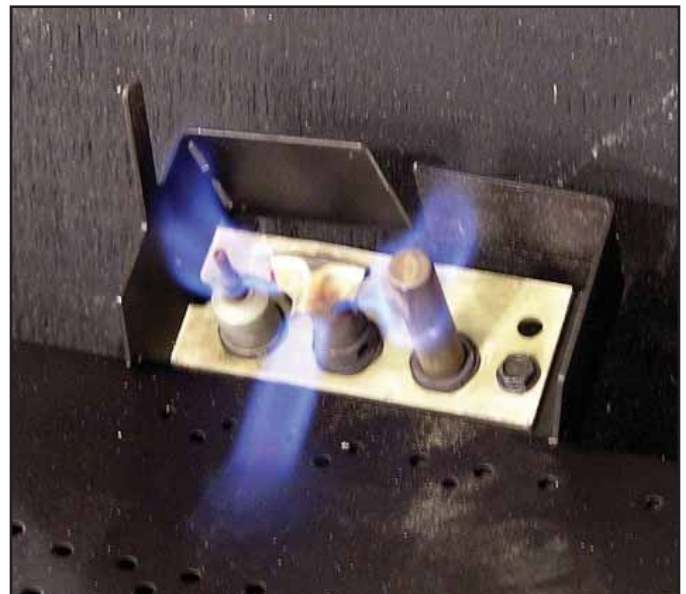
Figure 3.1 Standing Pilot Flame Patterns
