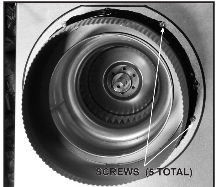
Figure 8A.9 Base Plate Fastened to Intake
