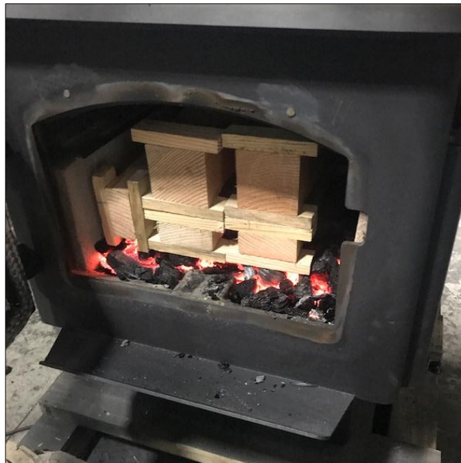
Typical Test Fuel Loaded in Test Stove
