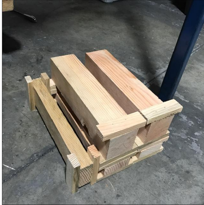
Typical Test Fuel Load Configuration
