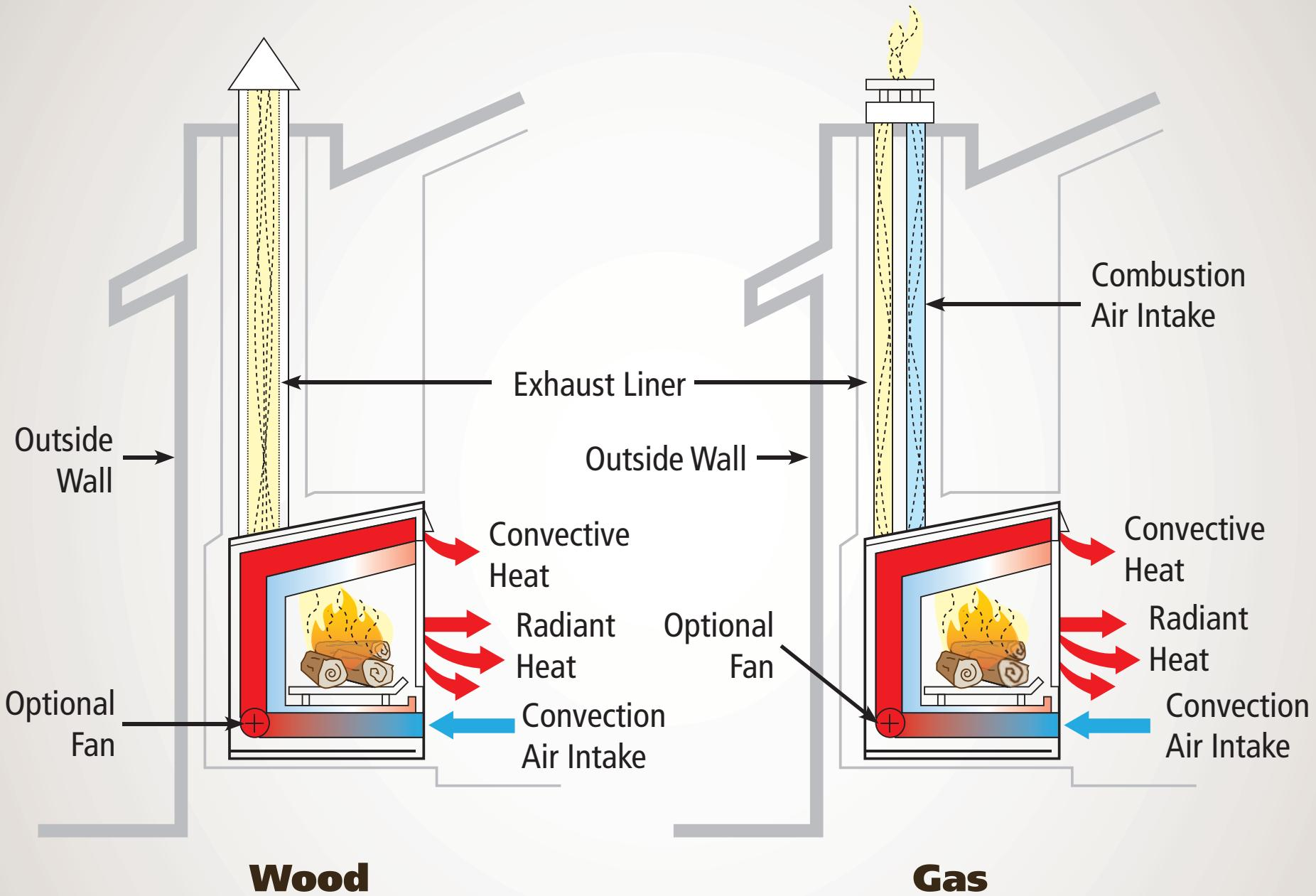
Each type of vent will use the existing chimney as the new vent passageway
