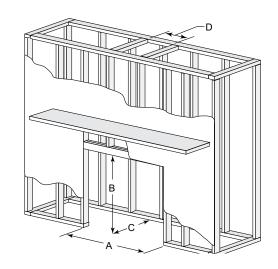
The rough framing dimensions shown represent the distance from stud to stud only and do not take into consideration the addition of drywall. Please refer to installation instructions for complete specifications and drawings when installing this product. Go to heatilator.com to download.
